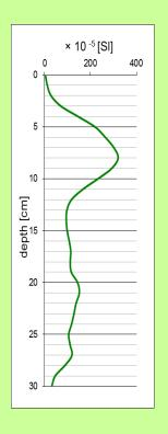
Laboratory measurement of  $\kappa$  value in the cores should be performed immediately, not later than 7 days from collection, during this time cores should be stored in a refrigerator.
