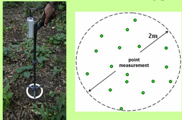
One measurement point consists of at least 11 individual measurements taken within a circle 2 m in diameter from the recorded GPS position
