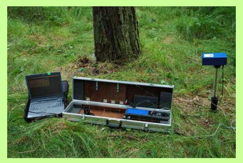
For in situ measurements, the diameter of the core probe must correspond to the diameter of the magnetic susceptibility meter.
